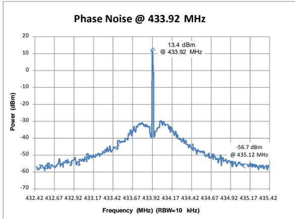
**Figure 3. Phase Noise,  $F_{RF} = 433.92$  MHz,
