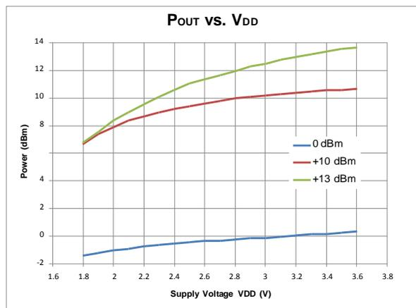
**Figure 8. Output Power vs. Supply
