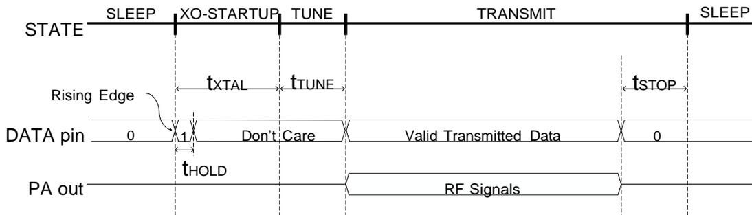
**Figure 16. Transmission Enabled by DATA Pin Rising Edge**
