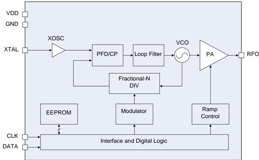
**Figure 11. RFM119ABW/RFM119ACW Functional Block Diagram**
