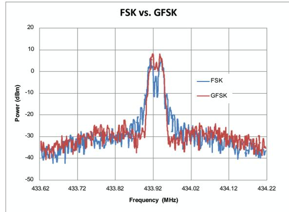
**Figure 6. FSK/GFSK Spectrum,
