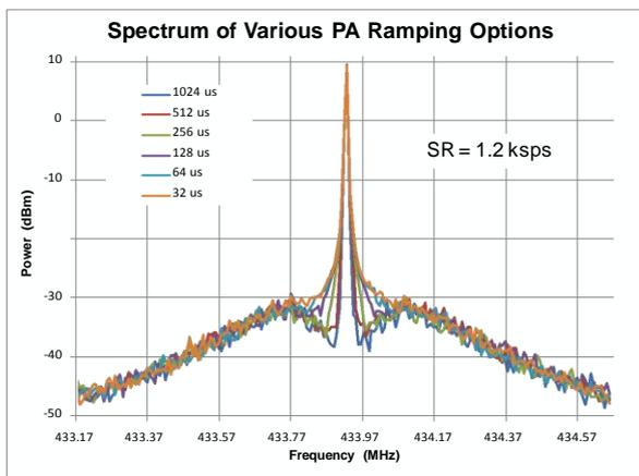
**Figure 7. Spectrum of PA Ramping,
