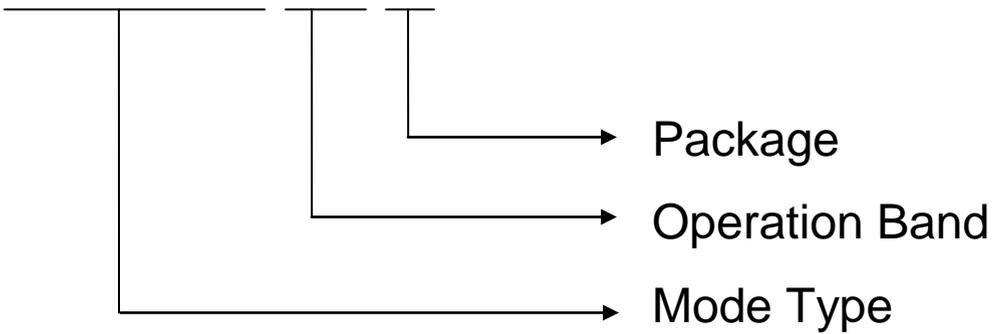
**P/N: RFM119ABW-433S2****RFM119ABW module at 433.92MHz band,SMD Package****P/N: RFM119ACW-868S2****RFM119ACW module at 868.35MHz band ,SMD Package**
